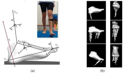
Figure 1 – (a) Experimental protocol and multibody model; (b) FEM model w/ contact forces and application points.
